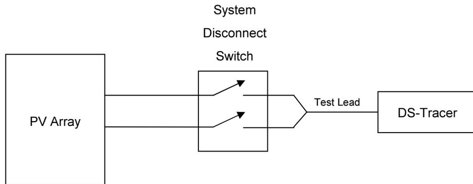
Figure 9. Use of PV system disconnect switch.
