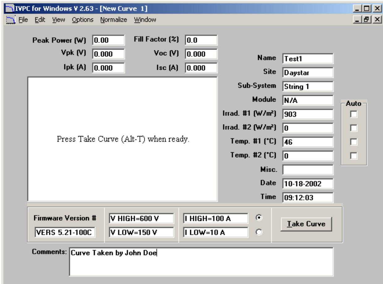
Figure 4. DS-Tracer is pre-charged and ready to immediately take the curve.
